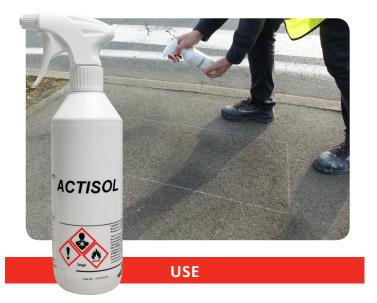
To be applied just before gluing ONLY on concrete surfaces (200-400g/m<sup>2</sup> depending on porosity), porous and coated natural stone (200g/m<sup>2</sup>).
